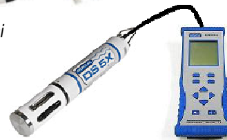
Hydrolab sonde and surveyor
